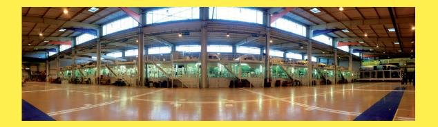
As a result of installing the MCE Pulse Line, 14 workstations are now available instead of the original 10 stations. The cycle jigs – an essential component of the system – are designed so that all work on the airplanes' interior can be carried out in line with the latest ergonomic and safety-related requirements.
