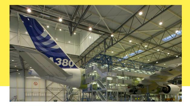
The furnishing platforms are designed to process the entire A380 family (700, 800, 800F, 900, and MAX). Each work area was designed, fabricated, installed, and commissioned after successful assembly at the client. The furnishing stations consist of different individual platforms and tools, all oriented in function to the assembly and logistics requirements for the A380 family.
