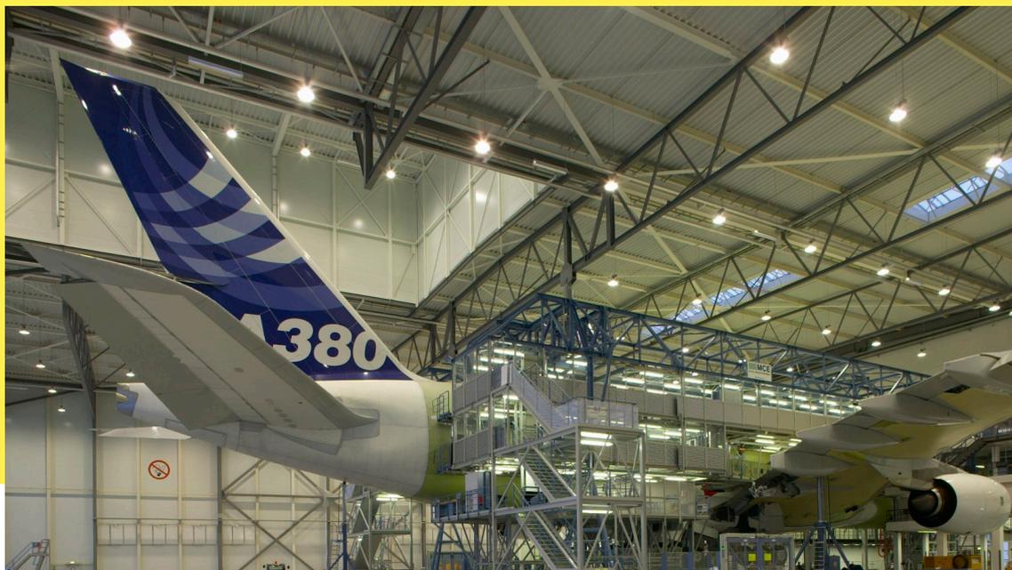
The furnishing platforms are designed to process the entire A380 family (700, 800, 800F, 900, and MAX). Each work area was designed, fabricated, installed, and commissioned after successful assembly at the client. The furnishing stations consist of different individual platforms and tools, all oriented in function to the assembly and logistics requirements for the A380 family.
