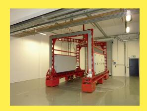
An adjustable tunnel geometry allows compact cars up to large transporters.
