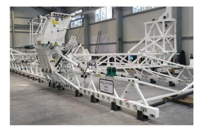
Toulouse - Blagnac, France - 2017 Airbus S.A.S. placed an order to MCE GmbH to deliver 6 Transport Jigs for the air transport of one pair full equipped A350XWB wings with the new Beluga XL transport freighter.
