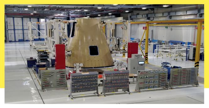
The two preparation stations are used to preassemble and predrill the frames for the later installation steps.
