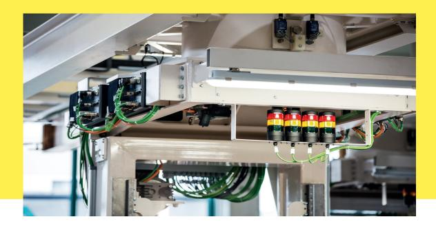
Every line consists of 6 stations. In the first station, the unequipped Pylon is loaded into the system and then automatically transferred by an overhead conveying system from station to station to comply with the equipment assembly. Every 6 hours, a new Pylon is loaded, and a finished Pylon gets out of each line. Moreover, the assembly requirement of two different Pylons (CFM, P&W) in each line is also fulfilled using a change adapter plate system.
